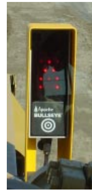
SurvCE, Tsunami, Dozer 2000, and GradeStar all can utilize optional Light Bar
